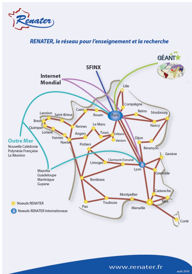
Fig. 1. The Renater5 Network provides 10Gb/s dark fibre links that Grid'5000 utilizes for its inter-site communication network (Courtesy of www.renater.fr)
